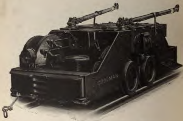
Crab Reel Driven from Locomotive Motor
